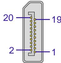
The following table indicates the pinout of the DisplayPort connector J9.
