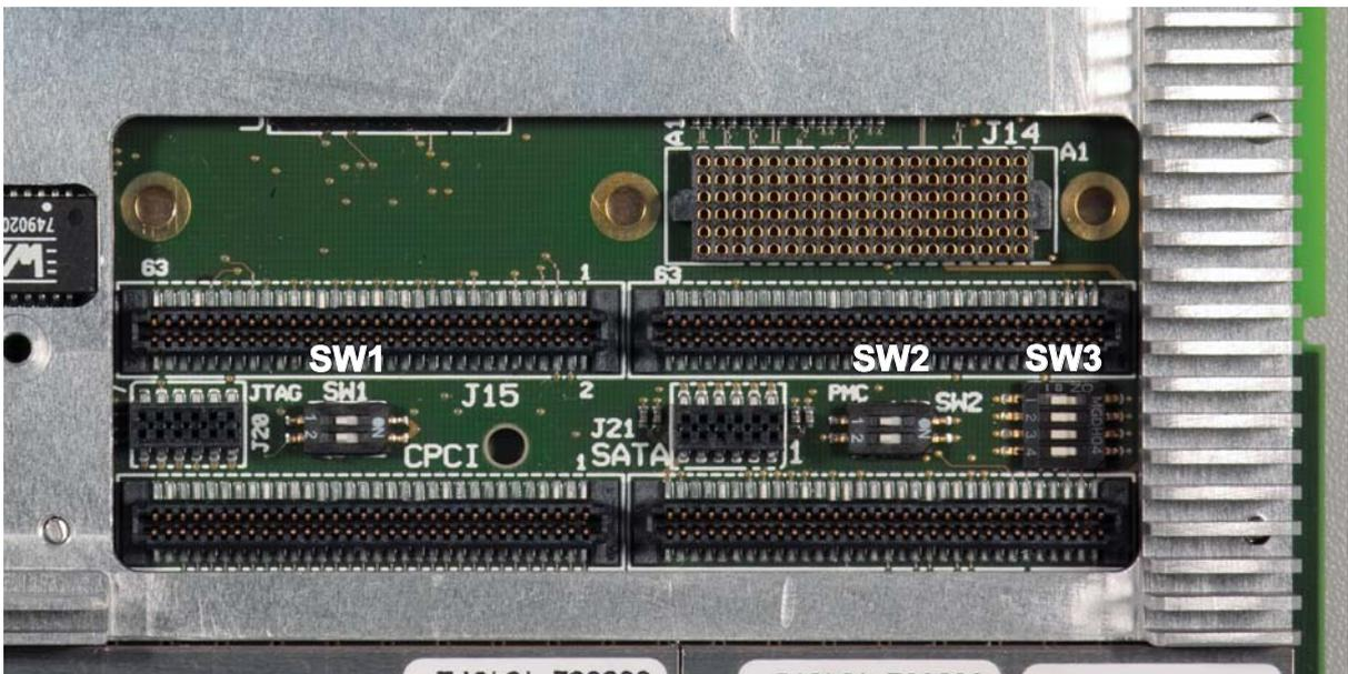
Table 4-1: DIP Switch SW1 for CompactPCI Interface Configuration
